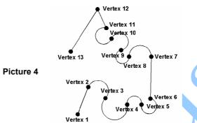
The vertexes 1, 6 and 12 start a line segment and the vertexes 2, 3, 4, 5, 7, 8, 9 and 10 start a circular arc. The below table show the characteristics of vertexes:
