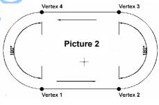
List like identify the coordinates of the vertexes: (10 x y). The dotted pair: (42 . x) show that the vertex start a line segment if x = 0.0 or a circular arc if x <> 0.0 (x<0 clockwise arc).
