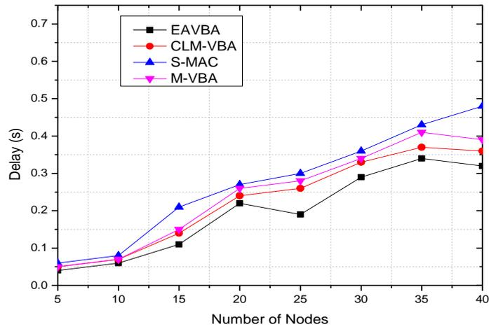
Figure 2: Performance of EAVBA compared with CLM-VBA, M-VBA and S-MAC in terms of delay
