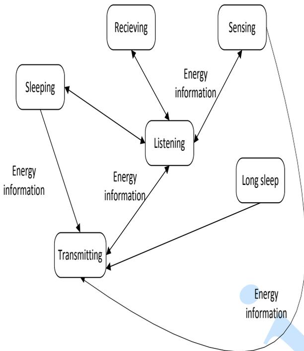
Figure 1: State Transition model for a node
