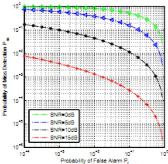
Figure 5: Roc Curves Over Nakagami Channel for M=10 Cooperating Detectors
