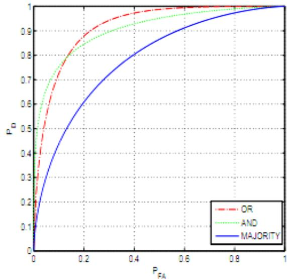
**Figure 3: ROC curves for OR, and AND majority fusion rules for  $m=10$  energy detectors**
