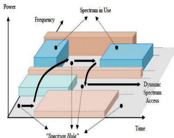
Figure 1; Spectrum Hole Illustration ([TMS09])
