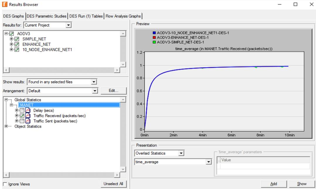
Fig 7. Traffic received at 10 Nodes
