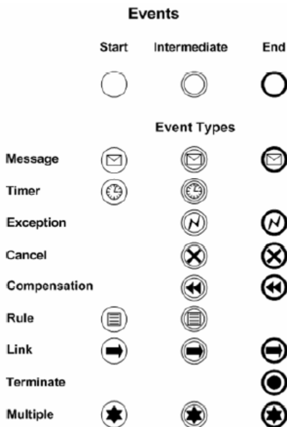
Fig. 1: Types of markers that can be added to BPMN core events [Whi05b]
