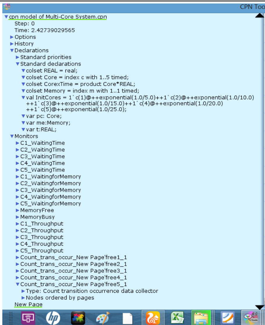
Figure 2: The Declaration of Color sets, Variables and Initial Parameters used in the Developed TCPN Model
