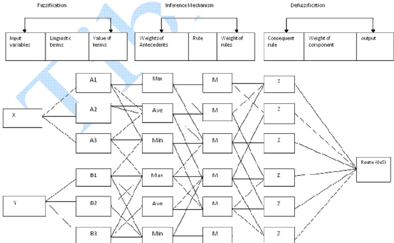
Figure 5: Architecture of Neuro – Fuzzy component of message routing (where M = multiply)
