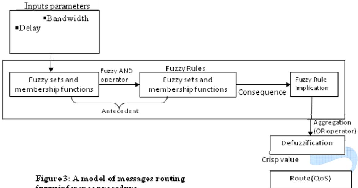
**Figure 3: A model of messages routing fuzzy inference procedure**
