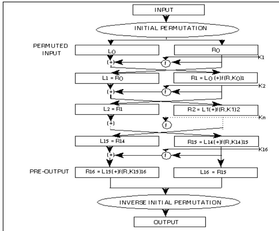
Figure 1. Enciphering Computation
