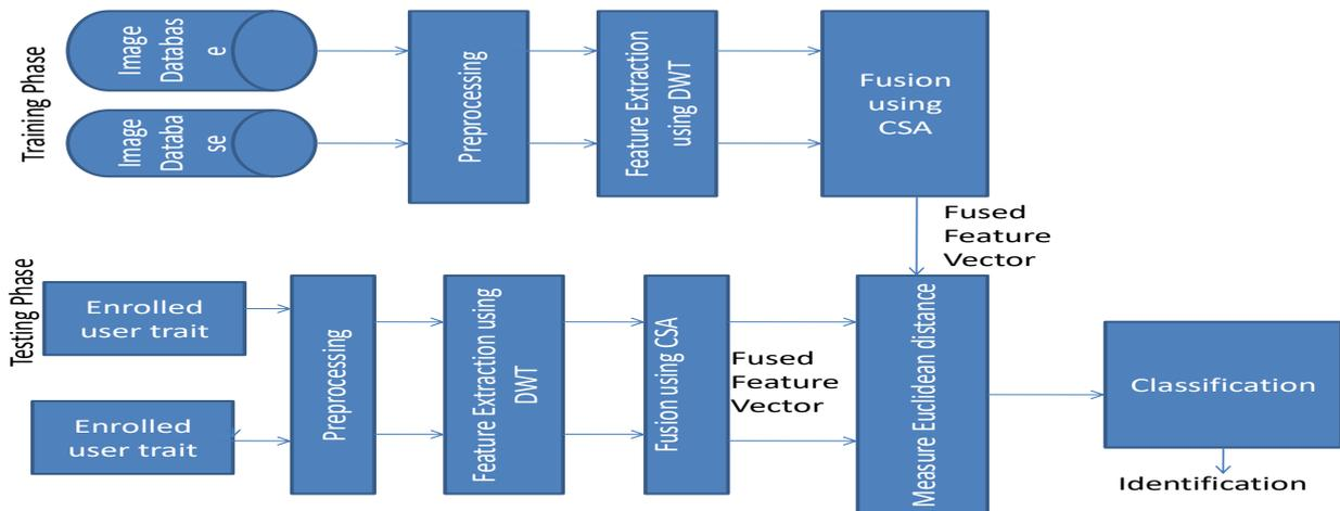
Figure 1: Process flow of a bimodal biometric system
