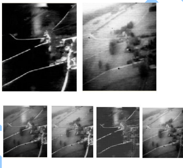
Figure 6 Experimental results of different fusion rules. (a) Image I (b) Image 2 (c) Averaging (b) Maximum (c) Minimum (d) PCA method
