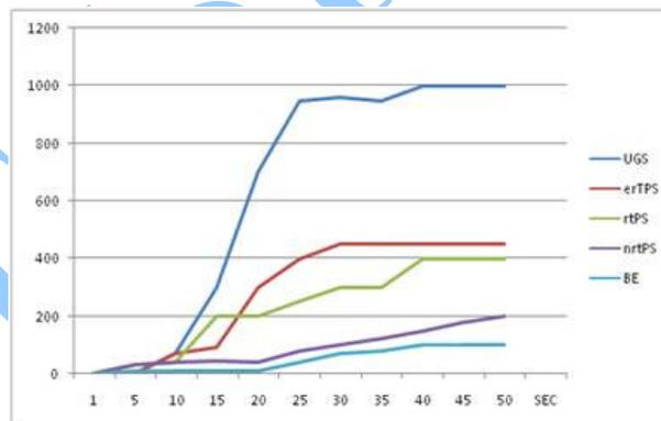
**Figure 5: Throughput achieved by each service type using queuing mechanism and bandwidth allocation algorithm**
