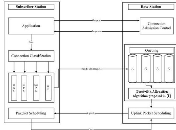
**Figure 2: Proposed Architecture for Bandwidth Allocation and Queuing Management**
