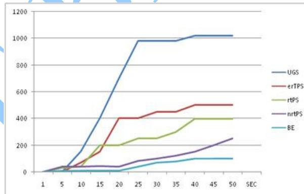
**Figure 4: Throughput achieved by each service type using queuing mechanism**
